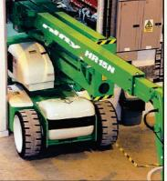
With more outreach than any other machine in its class and a base width of only 1.50m, the **HR15N** in one of the most effective and versatile self propelled platforms available.
