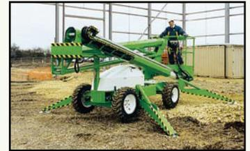
Rough terrain tyres as standard and the 4WD option allow the **SD170** to manoeuvre easily over a wide range of site conditions.
